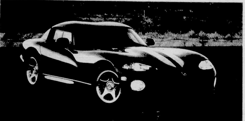
The 1996 Dodge Viper RT/10 will be the first domestically produced car to use Michelin Pilot MXX3 tires. The carcass, tread and compound of these tires are tuned to the new suspension package to provide more stability. The most notable construction change is a significant increase in sidewall stiffness. Reduced road noise and improved low temperature and wet traction objecties have been achieved along with substantial increases in cornering and braking traction. Wet cornering traction increased six percent in a standardized wet traction test. Peak lateral acceleration on the skidpad increased by over 5 percent. Stopping distance from 60 miles-per-hour is reduced by over 13 percent.
